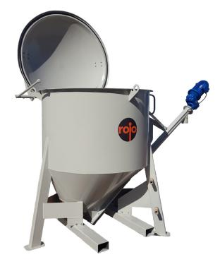
**MANEUVERABILITY:** The silo is easy to move around because it has its own removable forklift beams and it is also equipped with its own lifting handles for crane manoeuvrability. The 680kg weight and three legs are also enough to keep the silo steady during operating and the occasional vibrator usage.
